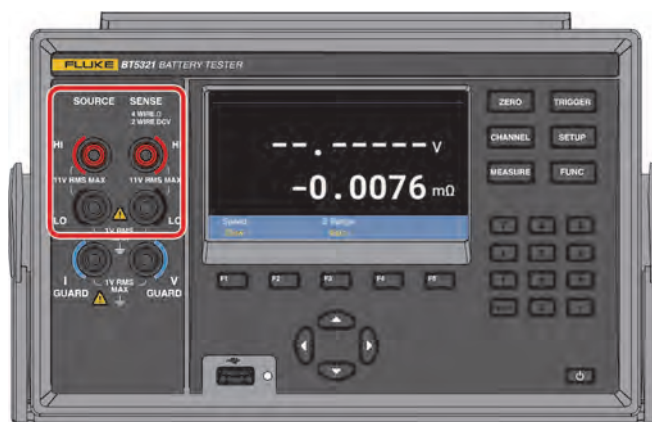
Figure 58. Measuring ACR, DCV and enclosure potential - front panel
