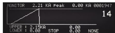
Monitor Screen – Shows weld current exceeding limit.
