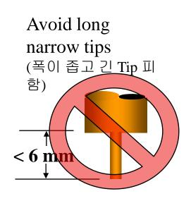
Electrode face after cleaning(Cleaning 후 전극 표면):
