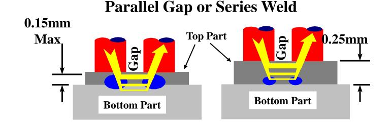
□ Limited to 0.15mm(.006in) thickness (0.15mm 두께로 제한)
