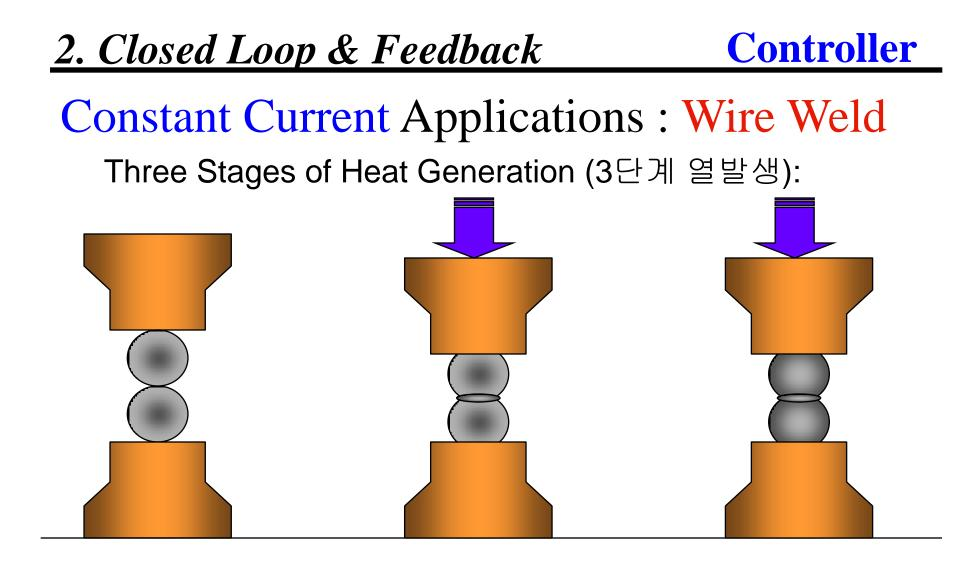
Beginning of Weld High Contact Resistance Wires Deform Reduced Contact Resistance
